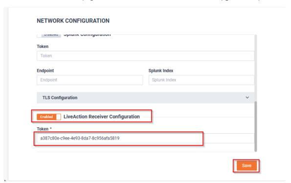
• Create a token for the LiveAction Receiver Configuration (if none is present).
